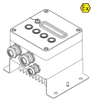
The LIM/DIS Ex-box is an electronic limiter for shutting down the connected electrical trace heating with lasting effect in case of overtemperature and is suitable for installation in potentially explosive atmospheres as well as inside or outside of buildings. The integrated control panel with display or the integrated bus interface can be used for programming and operation.
